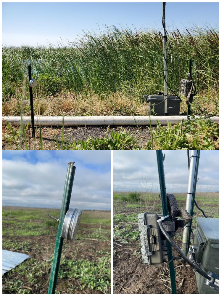
Figure 13: (Top) An example of a complete camera trap set up on Dutch Slough (top). An aluminum bait can secured to a T-stake with a nut and bolt (bottom left). Trail camera secured to T-stake with nylon strap and rubber gear tie and locked to the bait detector box with a python cable (bottom right).
